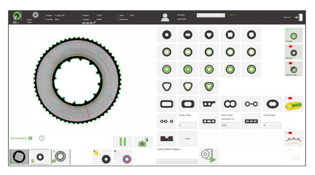
The measuring software VELOX evaluates obtained measuring results of the cross section measuring devices VCPX5 and AlphaOne with the latest generation of image processing algorithms.
